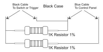
Normal Resistance: 2K  $\Omega$ ; Alarm Resistance: 1K  $\Omega$  Shorted Resistance: 0  $\Omega$ ; Open Resistance: Infinite  $\Omega$
